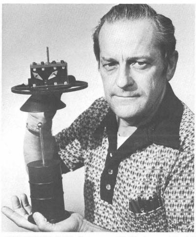
GENE ZUCUSKI (2323) displays a model of his "automatic hook." Hanging on the end of a single cable operating from a crane, the hook captures and releases ball-and-shaft-equipped containers simply and effectively. In plexiglass chamber above the guide ring, the capture and release levers are visible, the only moving parts within the device.
